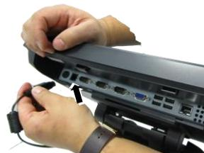
7. Tuck the extra cables inside the bottom I/O compartment, and then push back the cover to close it.
