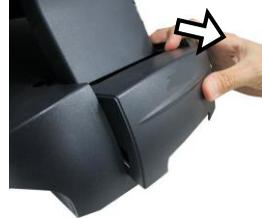
3. Pull outwards the locking levers with your forefingers and then remove the neck cover in the direction shown by the arrow.
