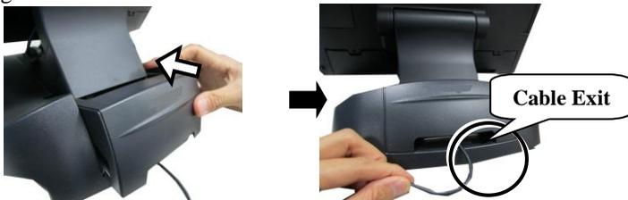
**CAUTION:** On doing insertion or extraction of a cable connector, please always hold the connector head itself instead of pulling the cable wire. Doing this could damage the cables and ports, which is considered as an artificial damage and is not covered by the warranty. The means of power cord should be connected to a socket-outlet with earthing connection.
