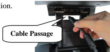
5. After tilting the screen all the way up, remove the bottom I/O cover to locate the bottom I/O plate.
